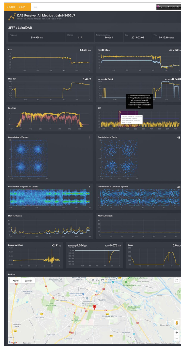
Fig. 4: The results of the DAB signal monitoring tests. DABRF received and recorded the signal from transmitter number three for analysis in the lab.
